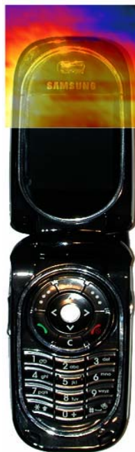
Figure 28 Sample H-field Scan Overlay
