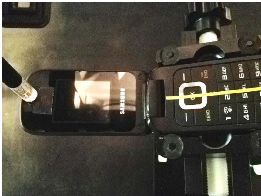
Figure 13-2 Test Setup for Wireless Device
