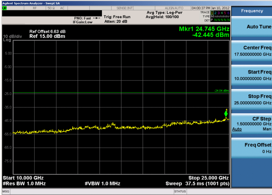
Plot 6-21. Conducted Spurious Plot (802.11b – Ch. 11)
