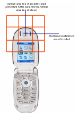
Figure 5.1 Wireless Device and Measurement Plane
