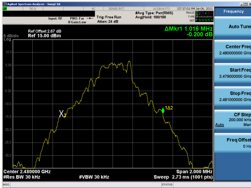
Plot 6-3. 20dB Bandwidth Plot (Bluetooth, 1Mbps – Ch. 78)
