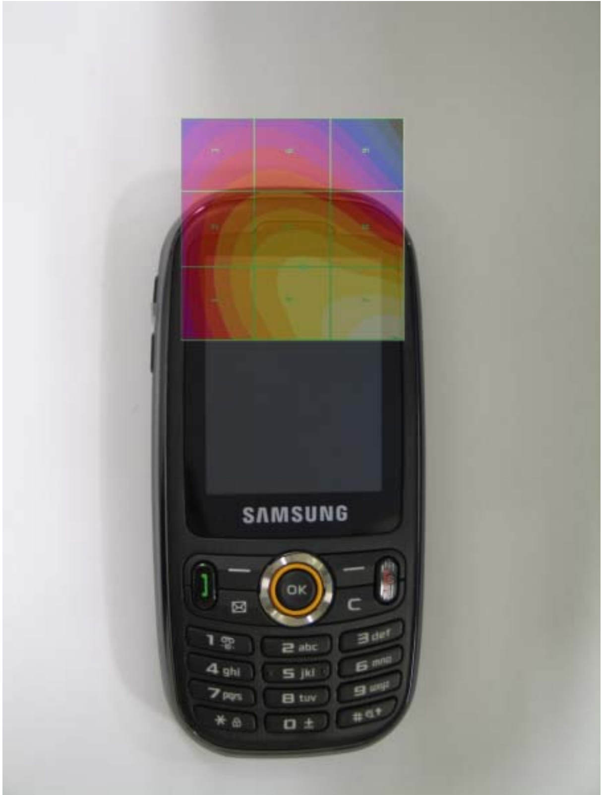
Scan overlay with actual device for GSM (H-field)
