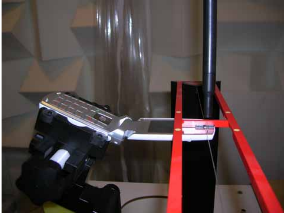
Figure 16-1 Ear Reference Point HAC Phantom Alignment
