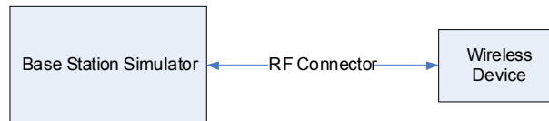
Figure 11-1 Power Measurement Setup
