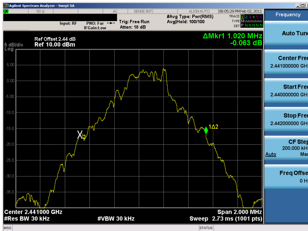
Plot 6-2. 20dB Bandwidth Plot (Bluetooth, 1Mbps - Ch. 39)
