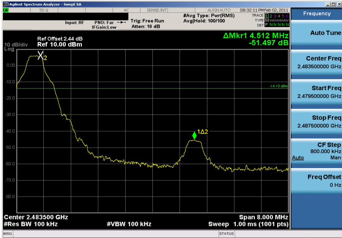
Plot 6-11. Band Edge Plot (Bluetooth, 1Mbps - Ch. 78)
