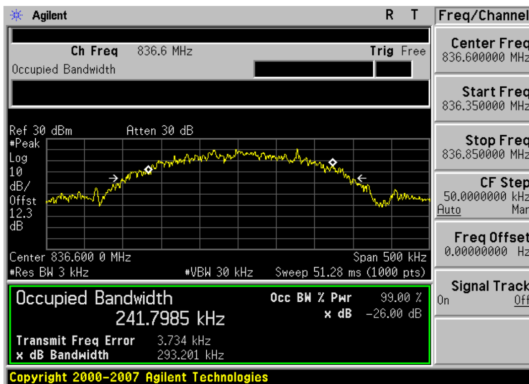
Plot 7-10. Occupied Bandwidth Plot (EDGE850 Mode – Ch. 190)
