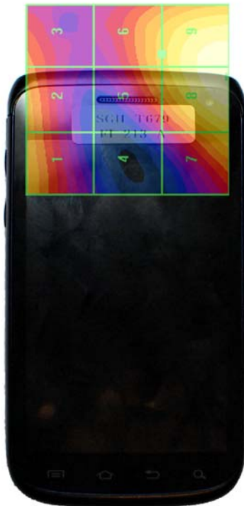
Figure 17-4 E-Field WD Scan overlay
