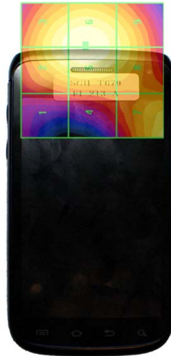
Figure 17-5 H-Field WD Scan overlay
