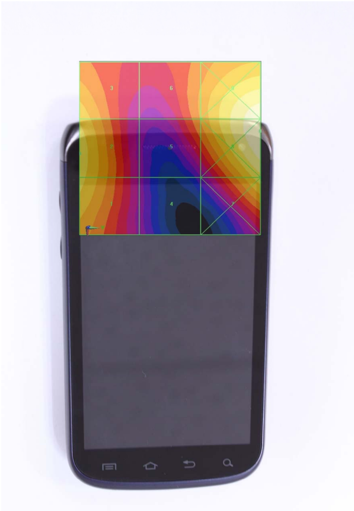
Scan overlay with actual device(E-field)
