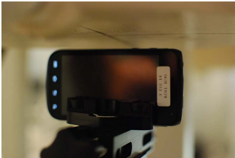
SAR Test Setup Photo 10: Left at 1.0 cm
