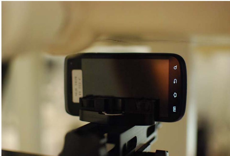
SAR Test Setup Photo 8: Right at 1.0 cm
