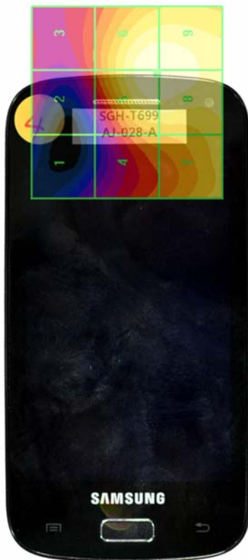
Figure 17-4 E-Field WD Scan overlay
