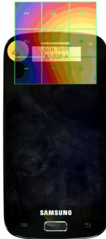
Figure 17-5 H-Field WD Scan overlay
