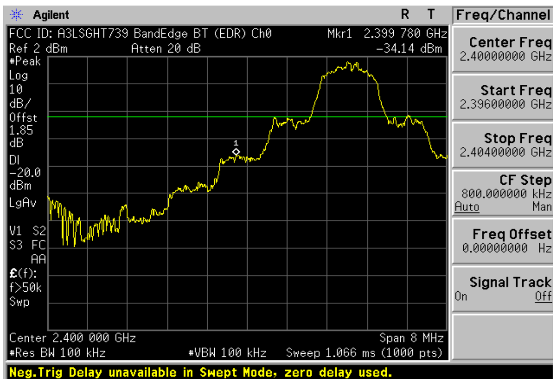
Plot 6-6. Band Edge Plot (Bluetooth 2.0 with Enhanced Data Rate – Ch. 0)
