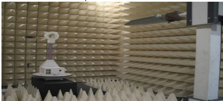
Figure2. Photograph of 3m Fully-Anechoic Chamber
