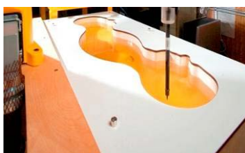
Figure 6-2 SAM Phantom with Simulating Tissue
