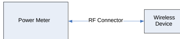
Figure 12-1 Power Measurement Setup
