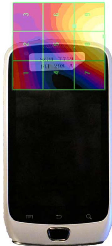
Figure 17-4 E-Field WD Scan overlay
