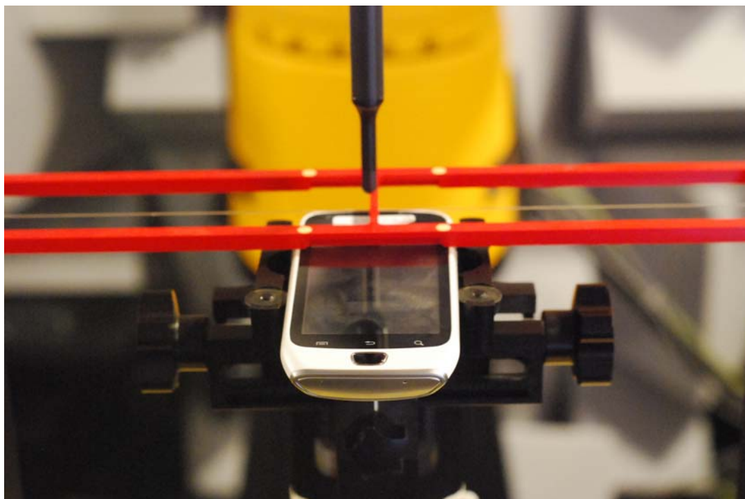
Figure 17-1 Ear Reference Point HAC Phantom Alignment
