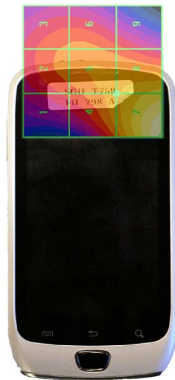
Figure 17-5 H-Field WD Scan overlay
