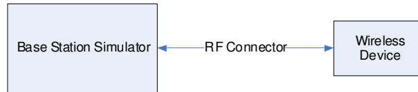
Figure 11-1 Power Measurement Setup
