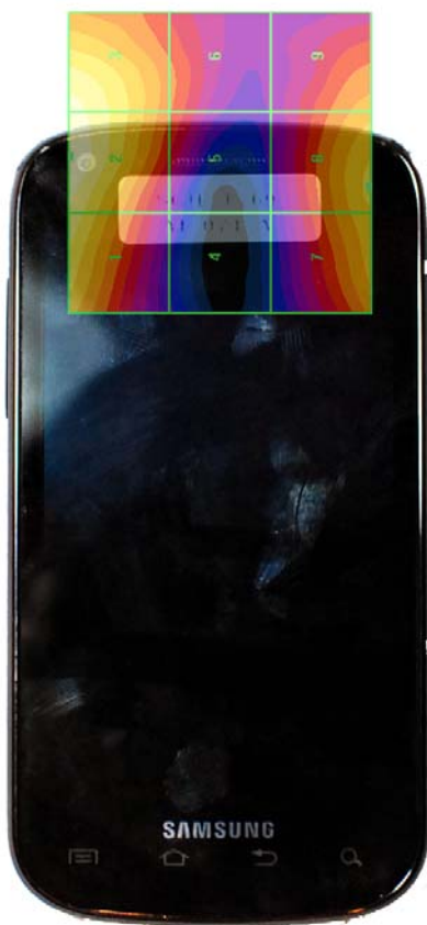
Figure 17-4 E-Field WD Scan overlay
