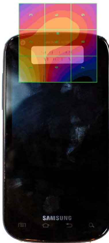
Figure 17-5 H-Field WD Scan overlay
