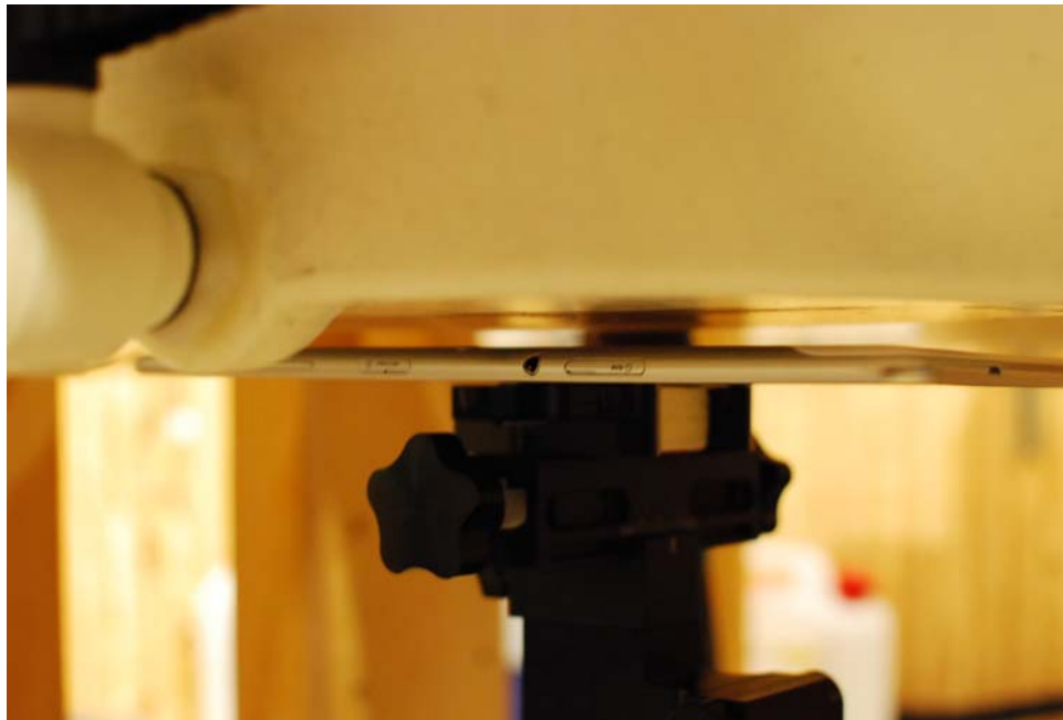
SAR Test Setup Photo 2: Back at 1.0 cm
