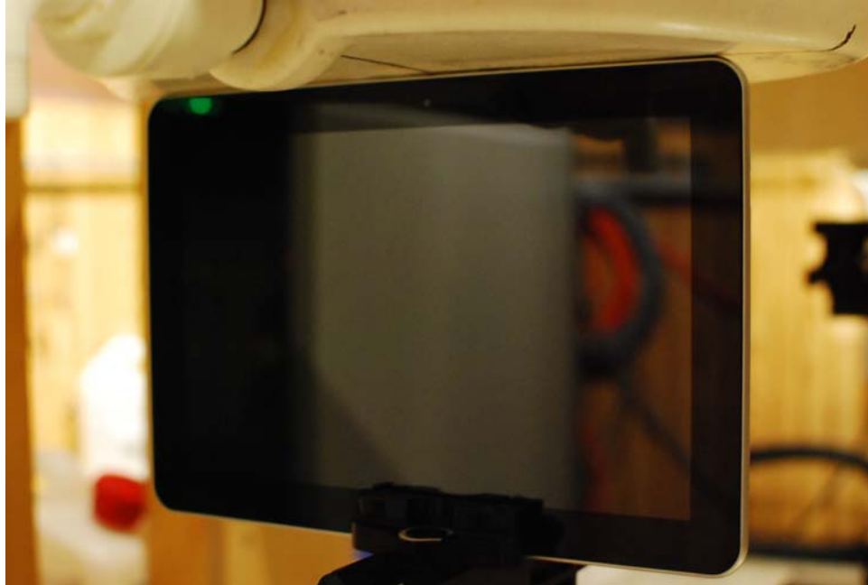
SAR Test Setup Photo 3: Top at 0.0 cm
