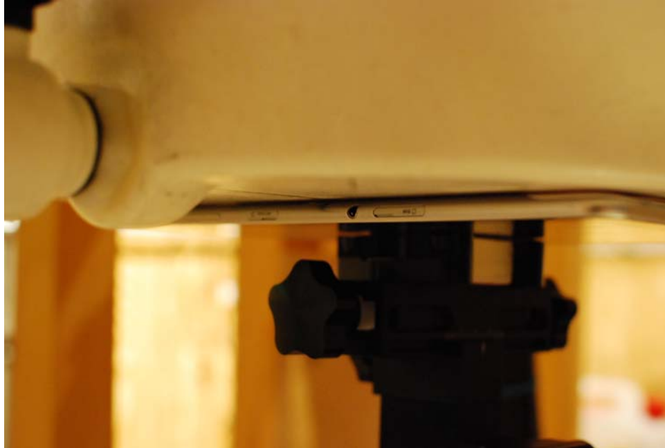
SAR Test Setup Photo 1: Back at 0.0 cm
