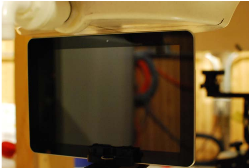
SAR Test Setup Photo 4: Top at 0.5 cm
