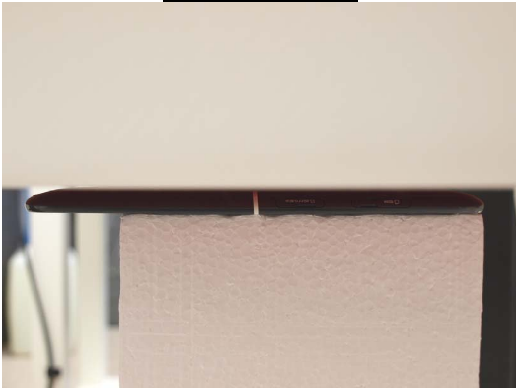
Rear/Base with 10 mm separation distance (Full Power)
