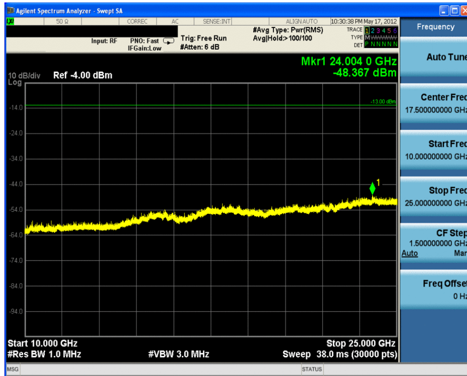
Plot 7-2. Conducted Spurious Plot (AWS WCDMA Mode – Ch. 1312)
