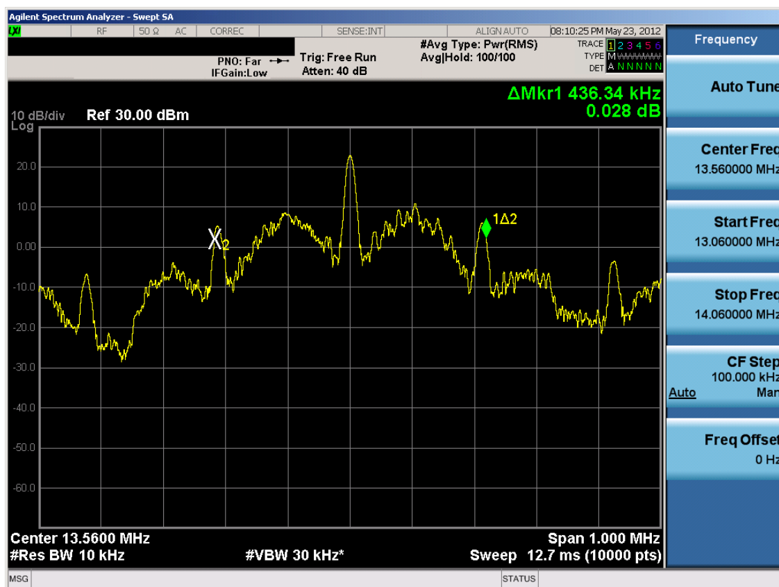
Figure 8-2. 20dB Bandwidth Plot
