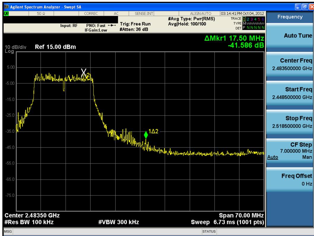
Plot 6-40. Band Edge Plot (802.11n (2.4GHz) – Ch. 11)
