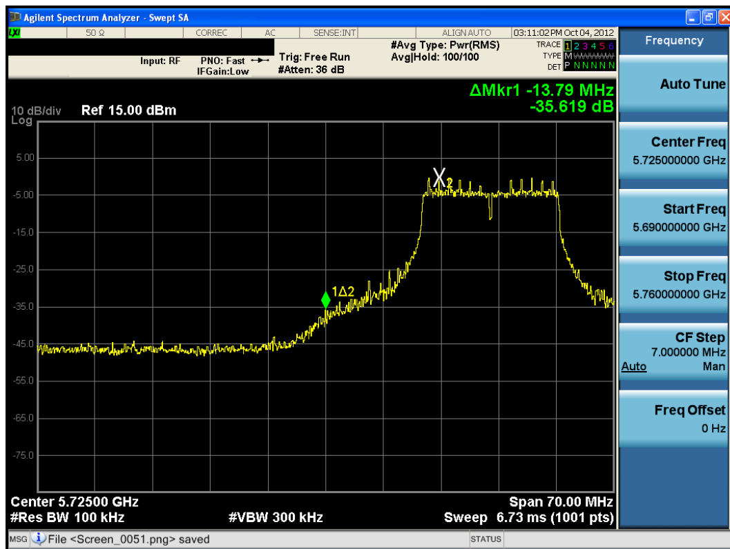
Plot 6-41. Band Edge Plot (802.11a – Ch. 149)
