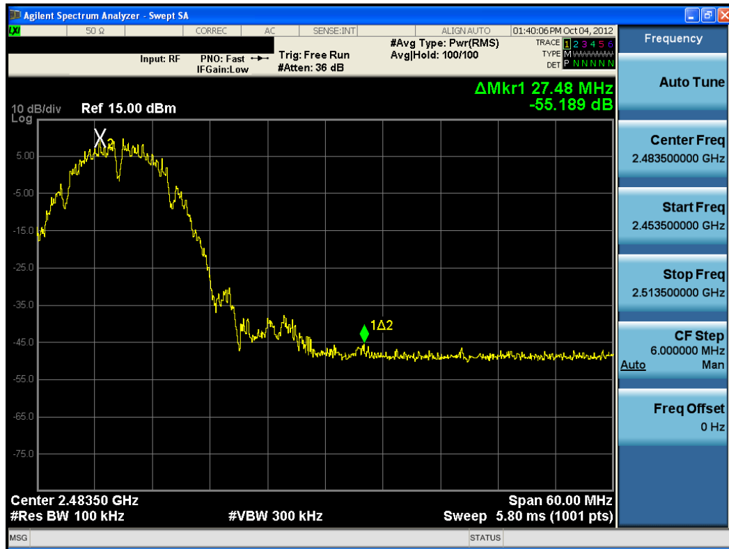
Plot 6-36. Band Edge Plot (802.11b – Ch. 11)
