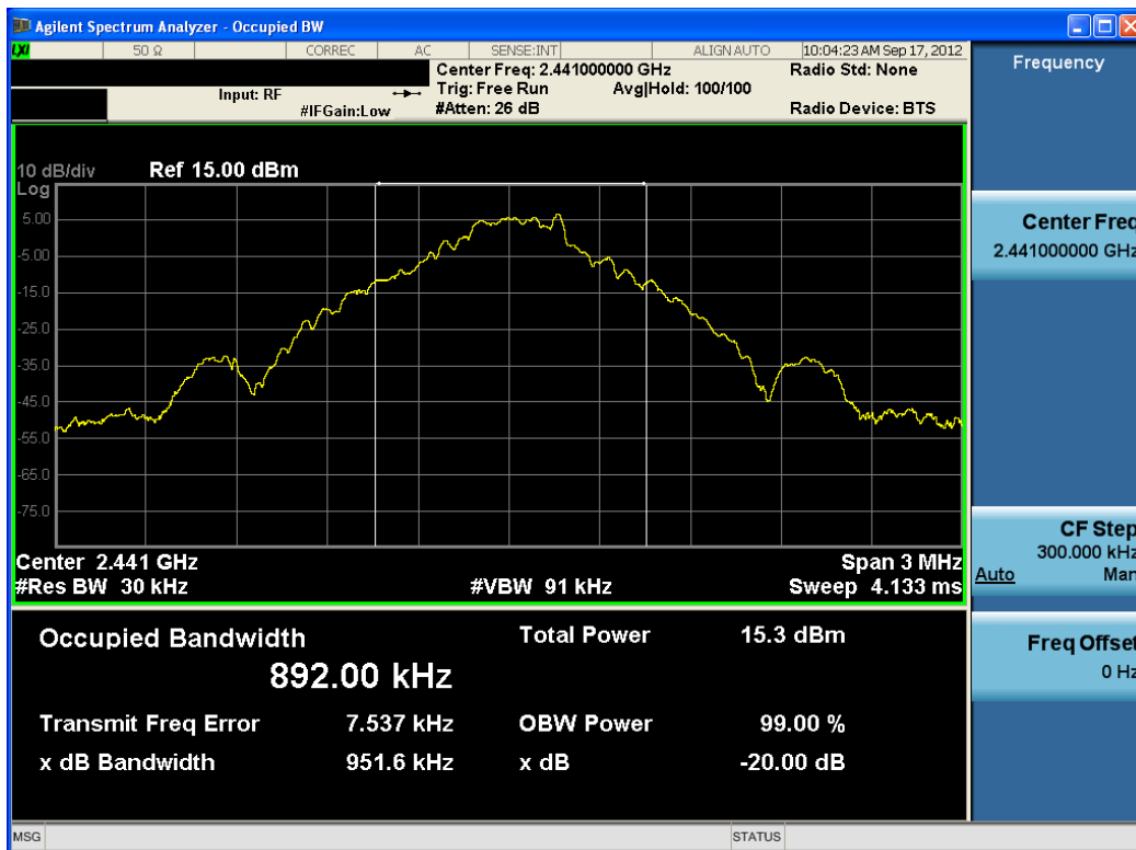
Plot 6-2. 20dB Bandwidth Plot (Bluetooth, 1Mbps – Ch. 39)
