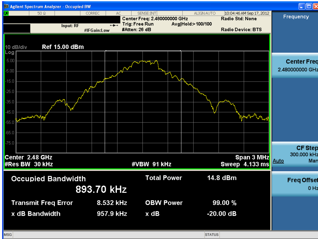
Plot 6-3. 20dB Bandwidth Plot (Bluetooth, 1Mbps – Ch. 78)
