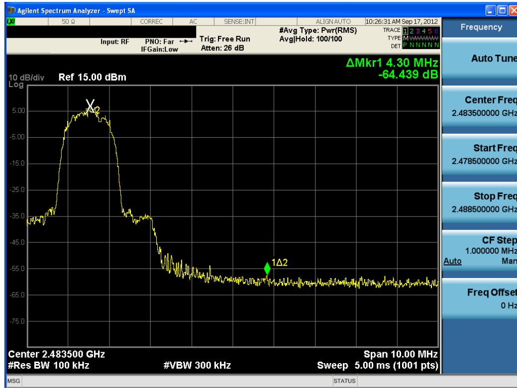
Plot 6-20. Band Edge Plot (Bluetooth with Hopping Disabled, 3Mbps – Ch. 78)
