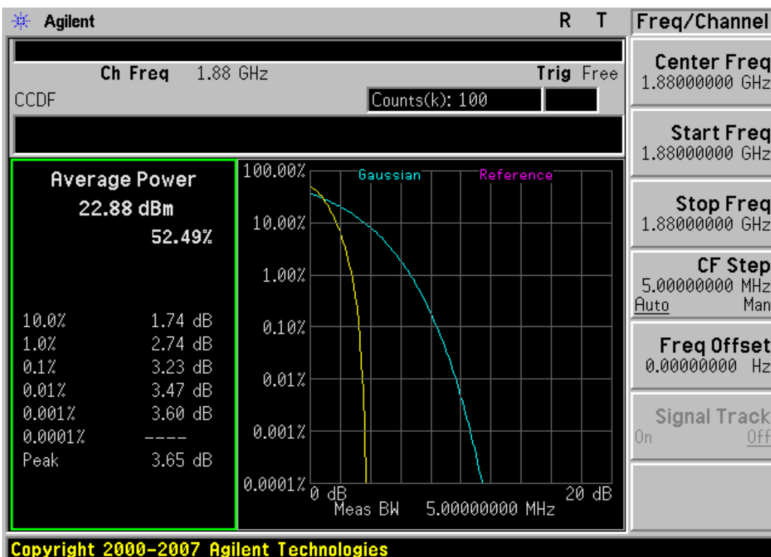
Plot 7-30. Peak-Average Ratio Plot (PCS WCDMA Mode – Ch. 9400)
