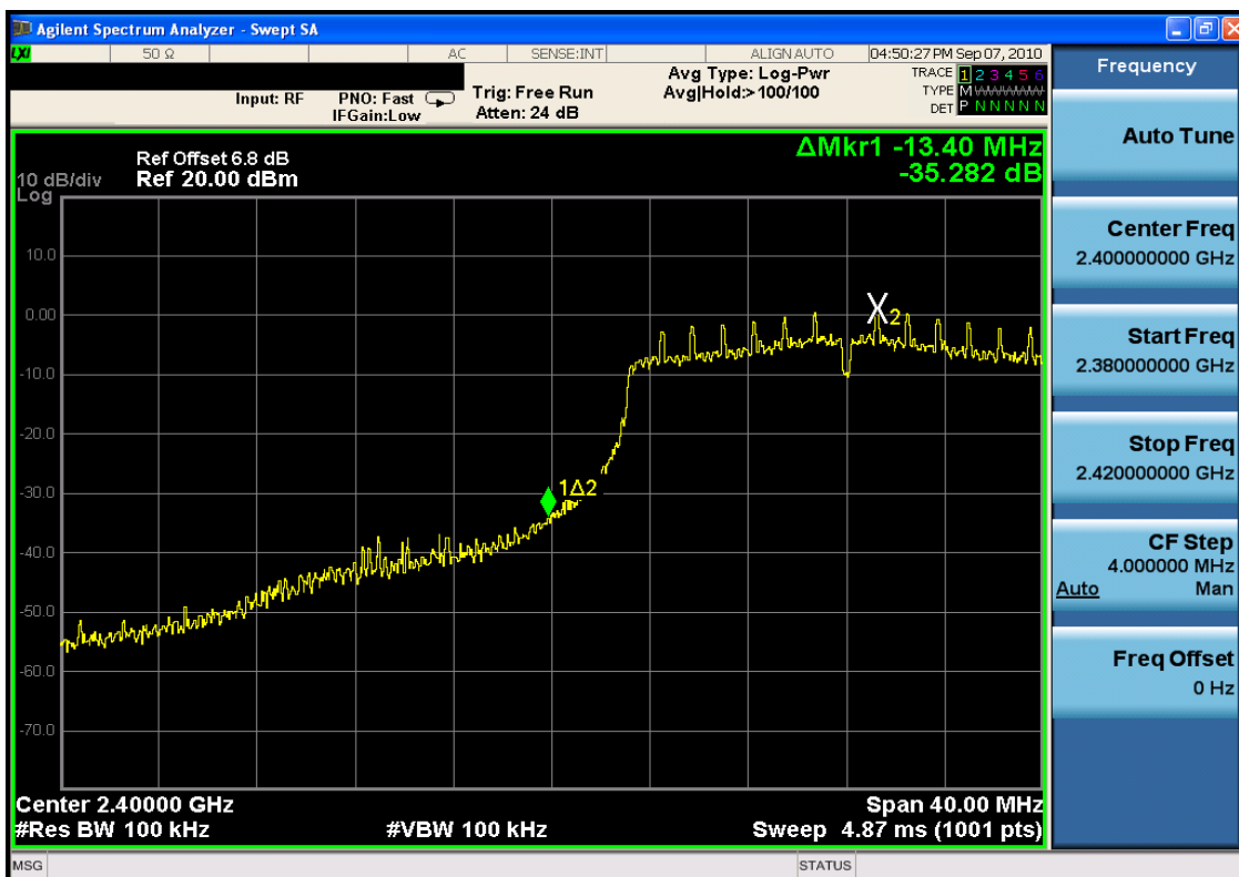
Plot 6-11. Band Edge Plot (802.11n – Ch. 1)
