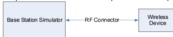
Figure 11-1 Power Measurement Setup
