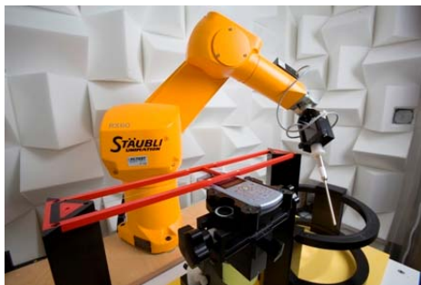
Figure 5-5 SPEAG Robotic System
