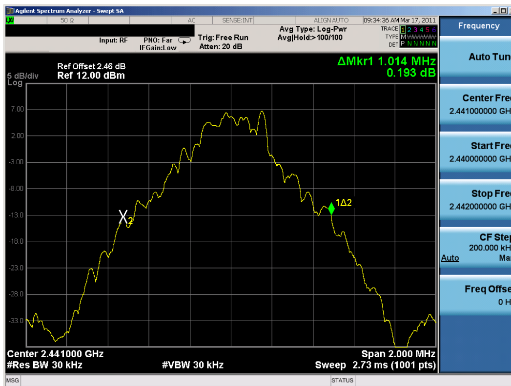
Plot 6-2. 20dB Bandwidth Plot (Bluetooth, 1Mbps - Ch. 39)
