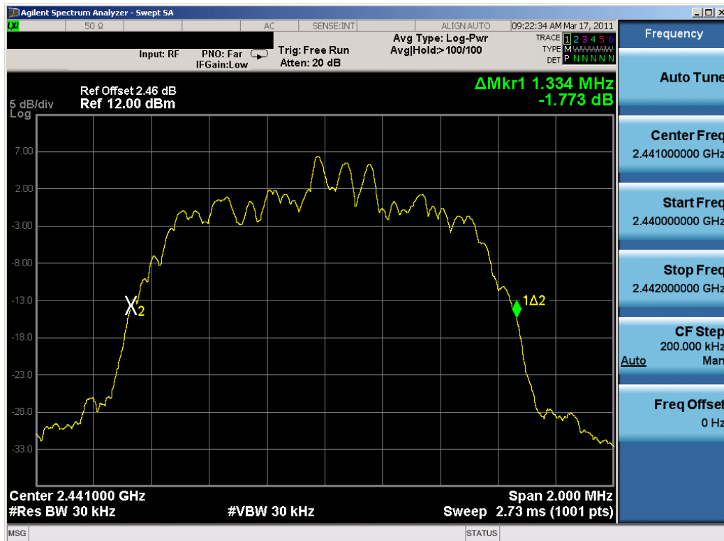
Plot 6-5. 20dB Bandwidth Plot (Bluetooth, 2Mbps – Ch. 39)
