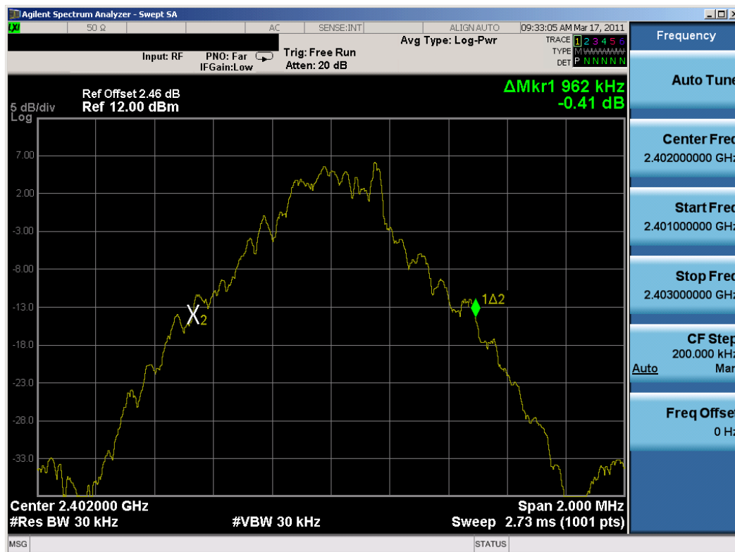
Plot 6-1. 20dB Bandwidth Plot (Bluetooth, 1Mbps - Ch. 0)
