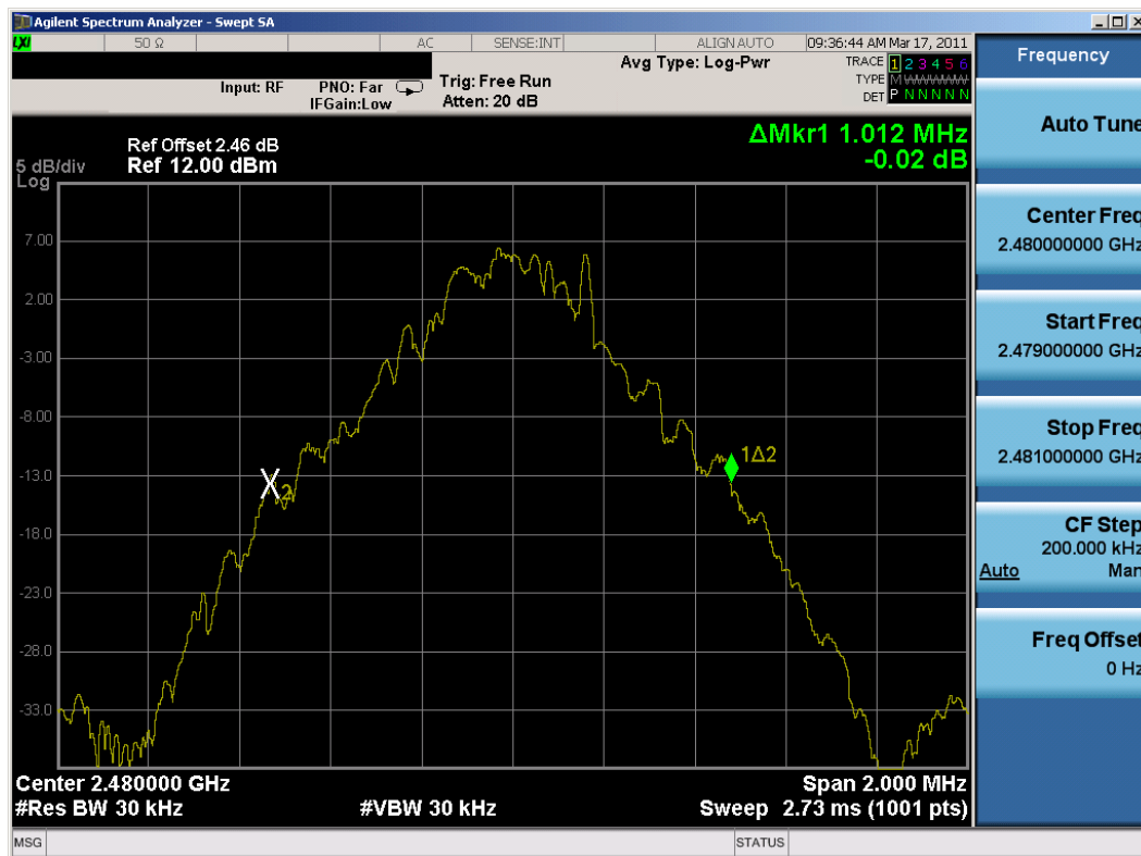
Plot 6-3. 20dB Bandwidth Plot (Bluetooth, 1Mbps – Ch. 78)
