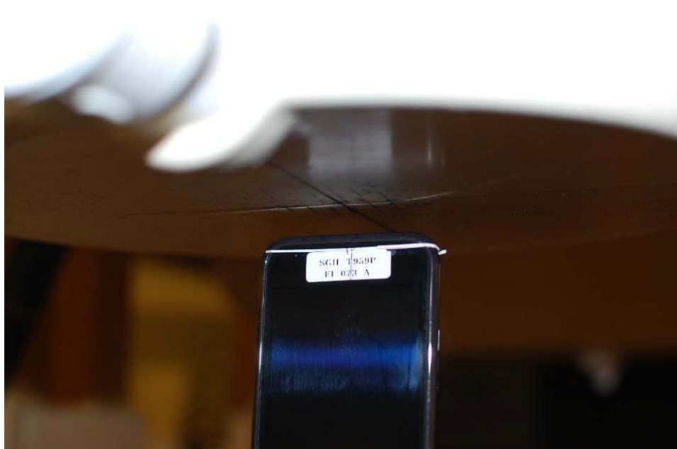
Figure 21-7 SAR Test Setup Photo 7 – Top at 1.0 cm
