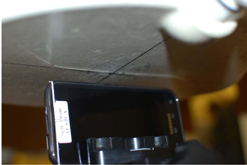
Figure 21-9 SAR Test Setup Photo 8 – Right at 1.0 cm
