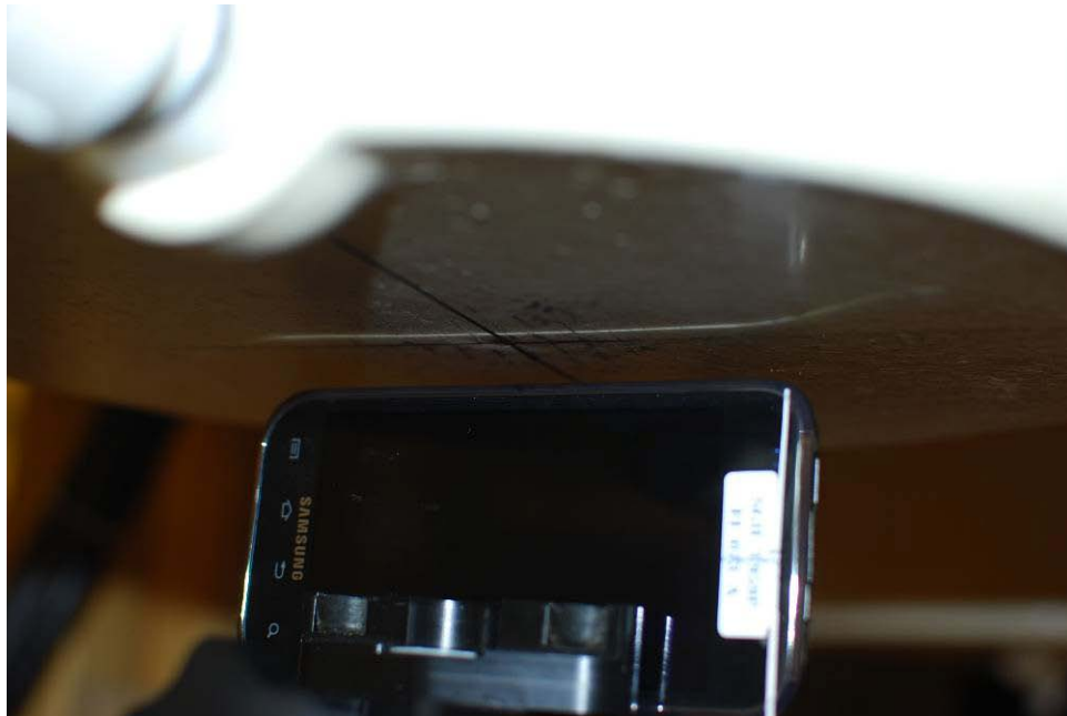
Figure 21-10 SAR Test Setup Photo 9 – Left at 1.0 cm
