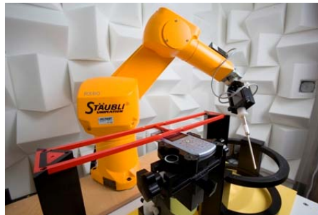
Figure 5-5 SPEAG Robotic System
