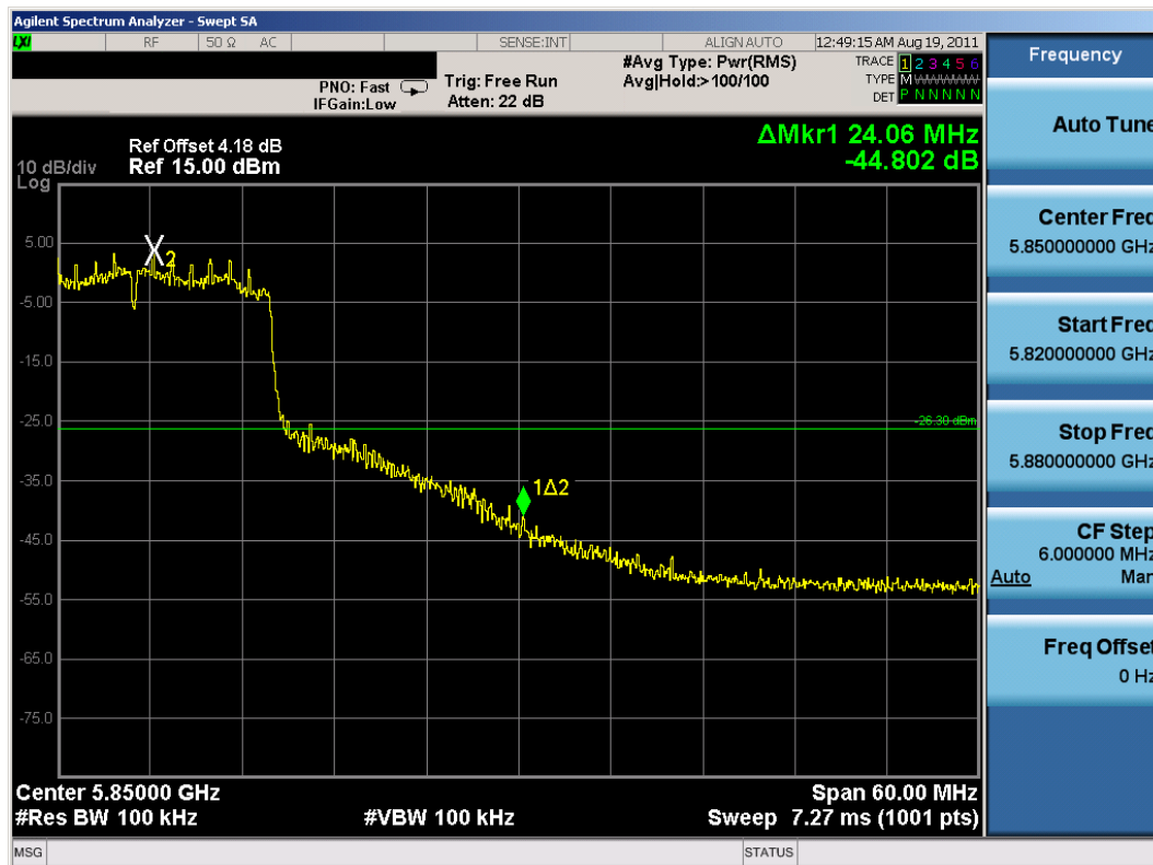
Plot 6-40. Band Edge Plot (802.11n (5.8GHz) – Ch. 165)
