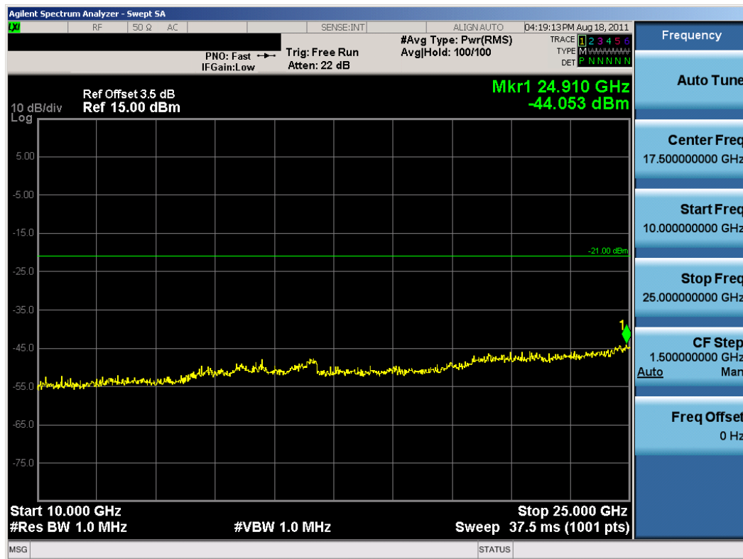
Plot 6-46. Conducted Spurious Plot (802.11b – Ch. 11)
