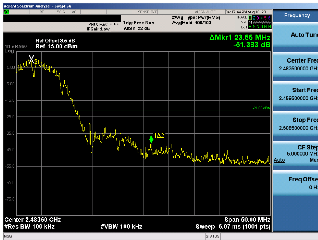
Plot 6-32. Band Edge Plot (802.11b – Ch. 11)
