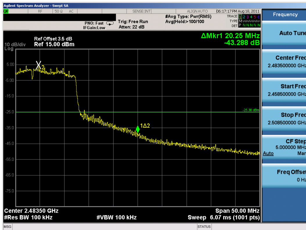
Plot 6-36. Band Edge Plot (802.11n (2.4GHz) – Ch. 11)
