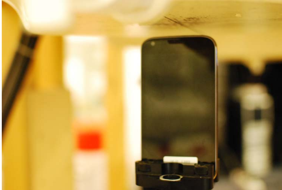
SAR Test Setup Photo 7: Top at 1.0 cm
