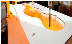
Figure 6-2 SAM Phantom with Simulating Tissue
