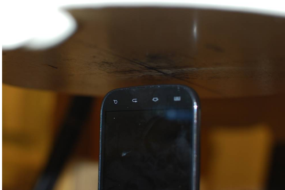
SAR Test Setup Photo 8 – Bottom at 1.0 cm
