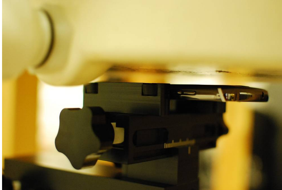
SAR Test Setup Photo 5 – Back at 1.0 cm
