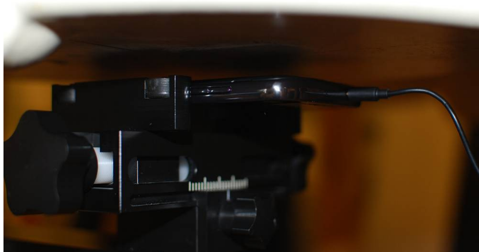
SAR Test Setup Photo 11 – Body-worn back at 1.0 cm
