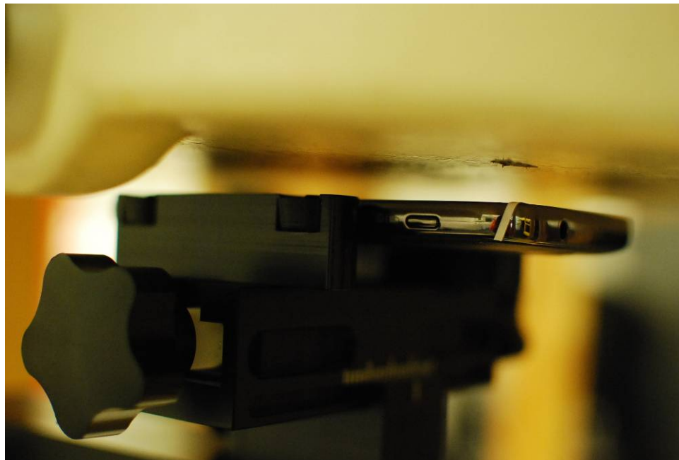
SAR Test Setup Photo 6 – Front at 1.0 cm
