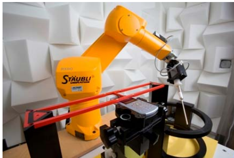
Figure 5-5 SPEAG Robotic System
