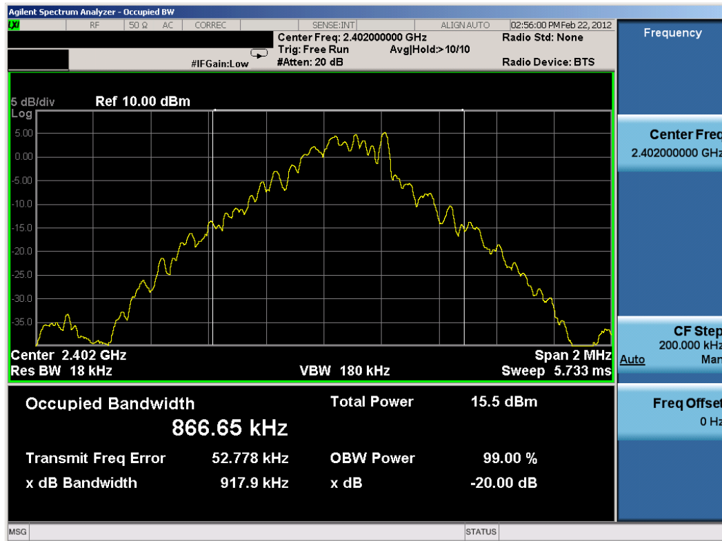
Plot 6-1. 20dB Bandwidth Plot (Bluetooth, 1Mbps – Ch. 0)
