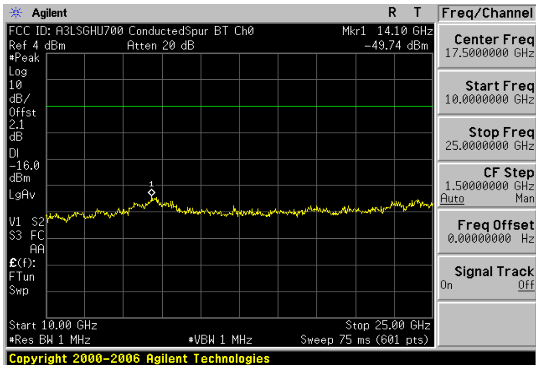
Plot 6-13. Conducted Spurious Plot (Bluetooth – Ch. 0)
