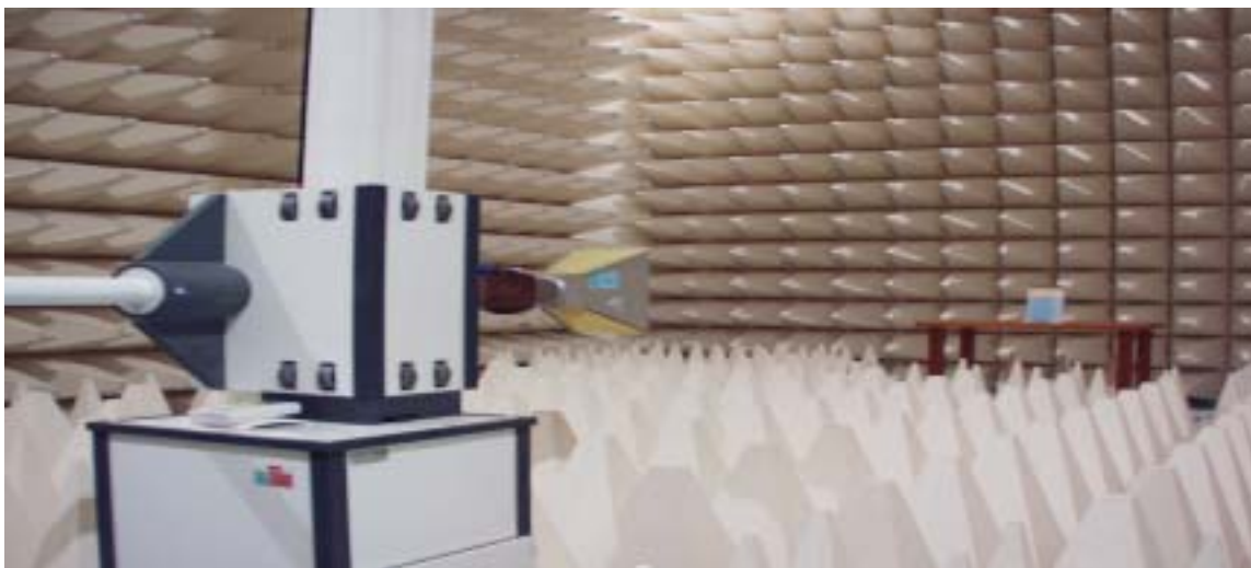
Figure2. Photograph of 3m Fully Anechoic Chamber
