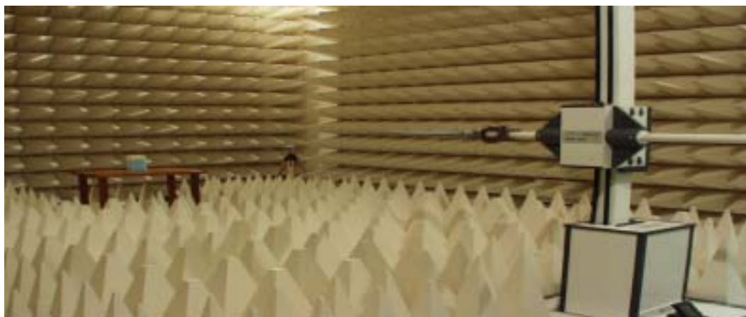
Figure2. Photograph of 3m Fully-Anechoic Chamber
