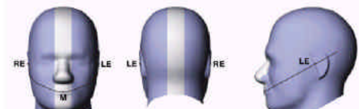
Figure 8.1 Front, back and side view of SAM Twin Phantom
