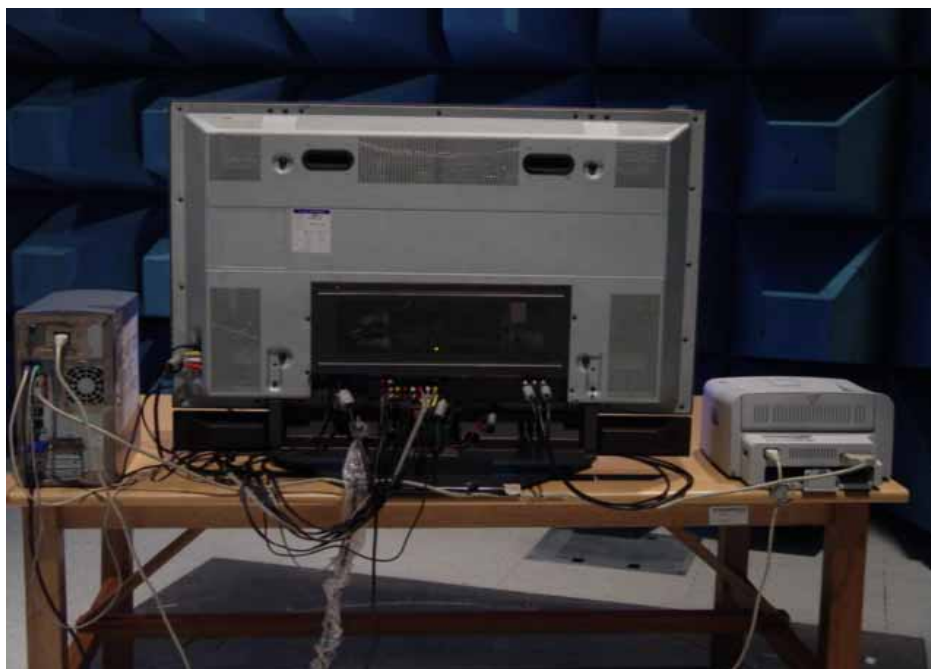
Picture 4. Radiated Emission (Rear)
