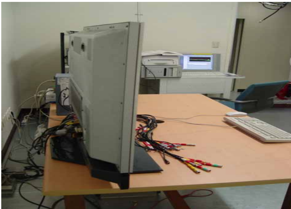
Picture 2. Conducted Emission (Side)
