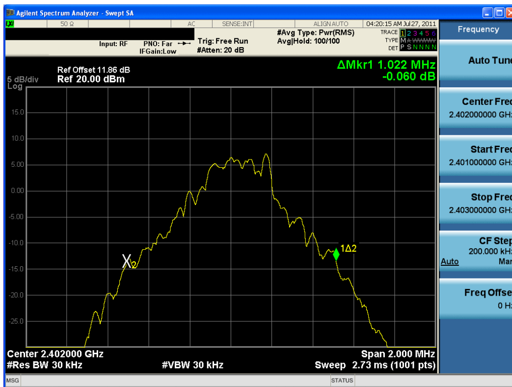
Plot 6-1. 20dB Bandwidth Plot (Bluetooth, 1Mbps – Ch. 0)
