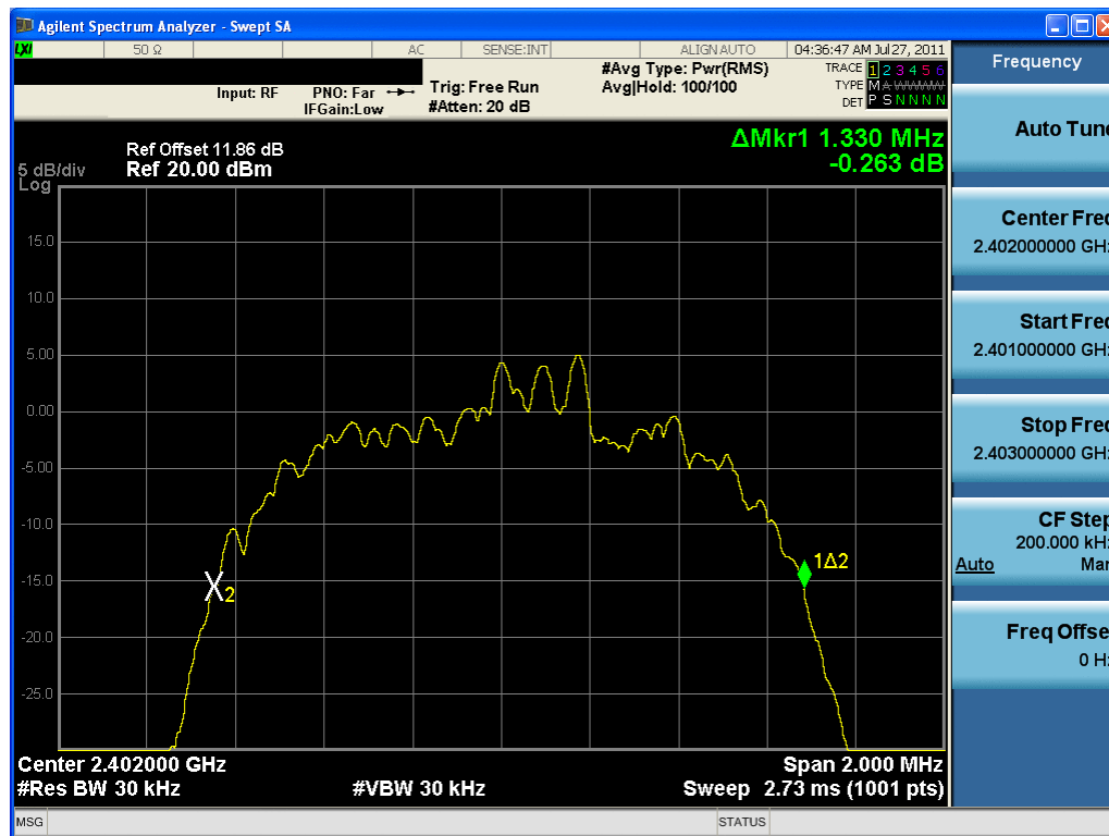
Plot 6-7. 20dB Bandwidth Plot (Bluetooth, 3Mbps – Ch. 0)
