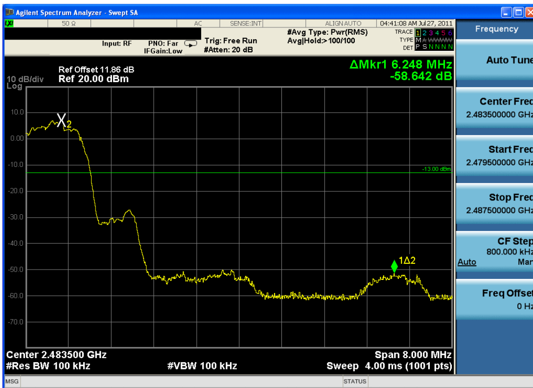
Plot 6-13. Band Edge Plot (Bluetooth, 3Mbps – Ch. 78)
