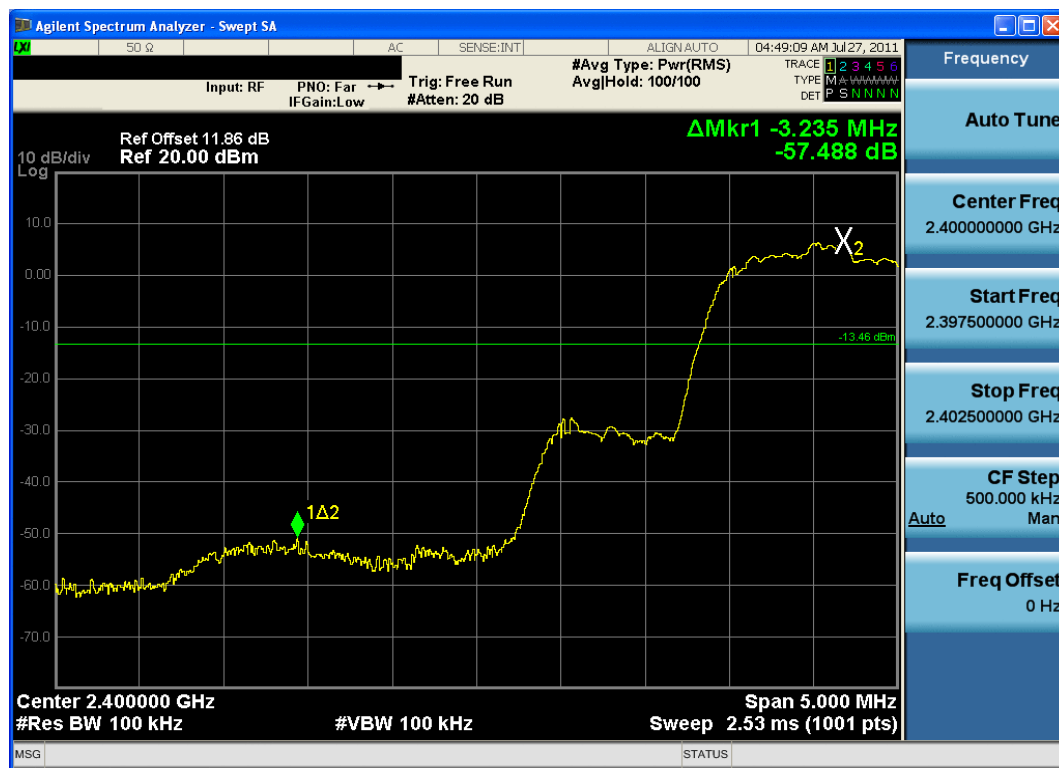
Plot 6-12. Band Edge Plot (Bluetooth, 3Mbps – Ch. 0)
