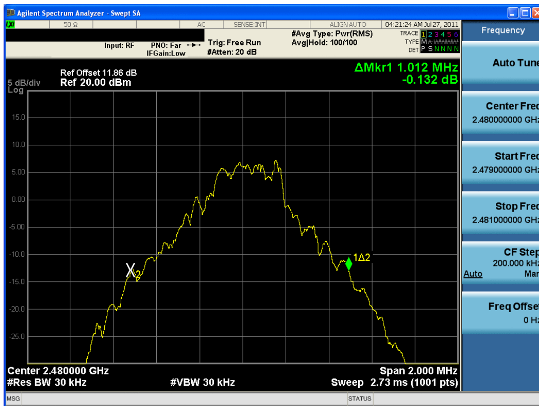
Plot 6-3. 20dB Bandwidth Plot (Bluetooth, 1Mbps – Ch. 78)
