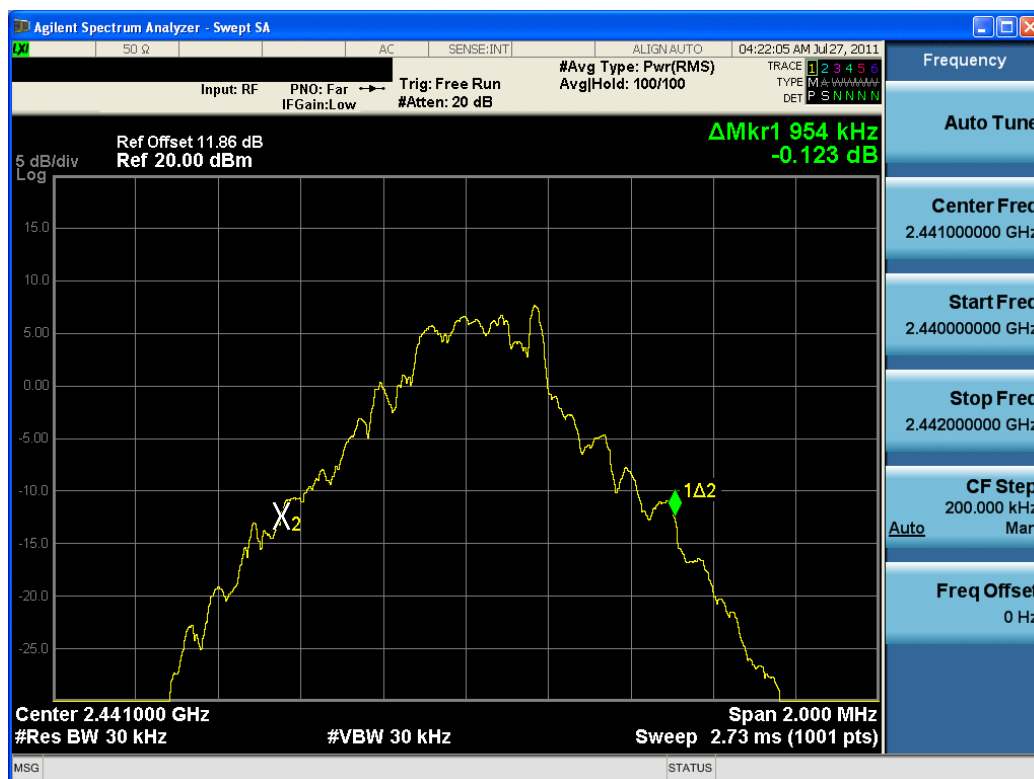
Plot 6-2. 20dB Bandwidth Plot (Bluetooth, 1Mbps – Ch. 39)
