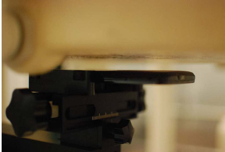
SAR Test Setup Photo 5 – Back at 1.0 cm
