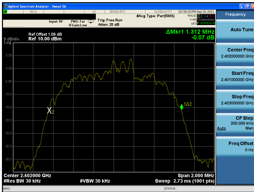
Plot 6-7. 20dB Bandwidth Plot (Bluetooth, 3Mbps – Ch. 0)
